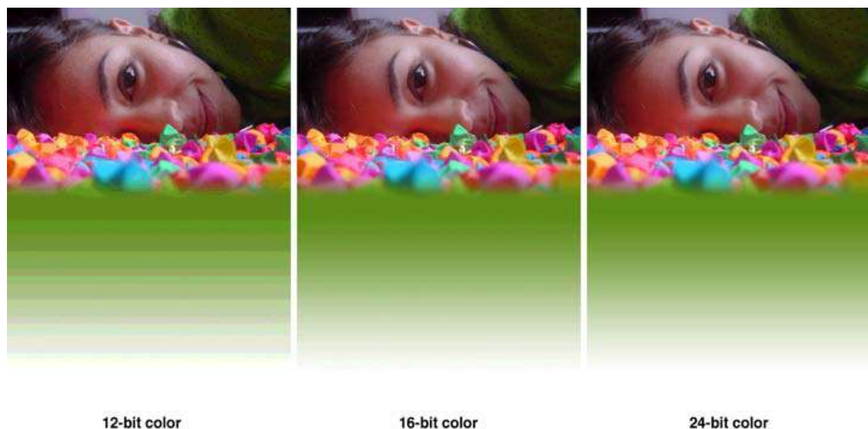
Figure 8-10. An example of different levels of posterization that can occur across multiple device colorDepths
