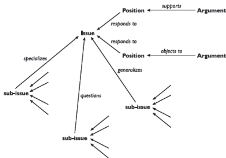
Figure 6.8 The structure of a gIBIS design rationale
